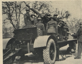
THE MOBILE 3-IN. ANTI-AIRCRAFT GUN, although not so well known as the 3.7, is a very effective weapon against high-flying planes. Its ceiling is 25,000 ft. and a 16-lb. shell is used. On left—A head-on view of a modern howitzer.
